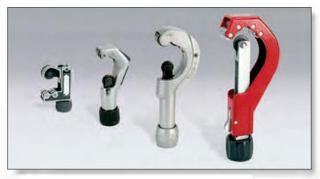
These tubing cutters are made from a high strength alloy; all feature rollers that are grooved which allows close to flare cuts. Some models have an enclosed feed screw which helps prevent clogging. Units are designed to cut soft copper, aluminum, brass and plastic tubing.
